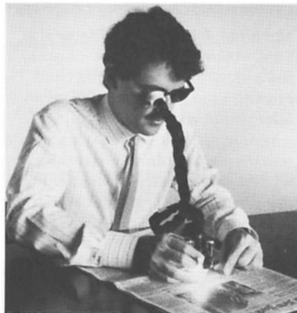
Figure 15. The fiberscope in use. The user scans the objective end over the page while looking through the eyepiece. A built-in battery-powered lamp illuminates the page.
