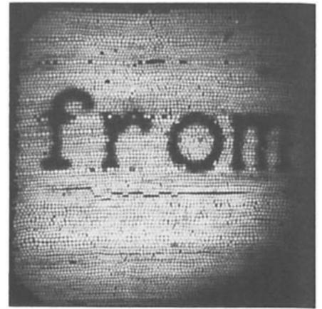
Figure 16. A view through the fiberscope. The honeycomb appearance is due to the individual optical fibers.
